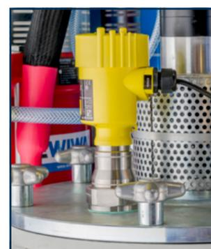
Radar sensors for level control
