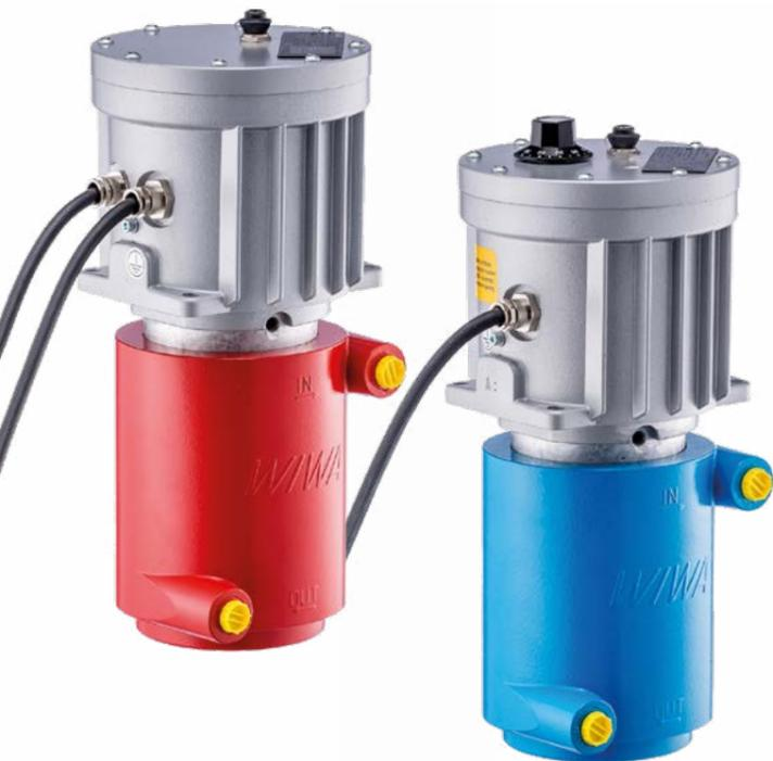
The WIWA material fluid heater with ATEX approval is the optimal addition for cold working environments. It ensures a constant temperature of the injection materials and can bring the container to be processed up to temperature by means of optional circulation. If required, heat can be used to the material to a shorter reaction time and thus accelerate the injection process.
