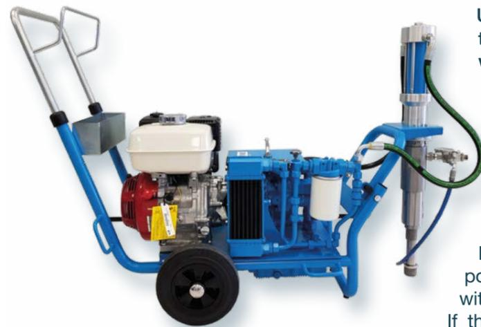
Unlike pneumatically or electrically driven pumps, the gas-powered WIWA HYDRO PX G operates with an independent power source, making it easy to maneuver over any terrain.
